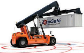
Large vehicles such as reach stackers can be fitted with multiple detection zones to cover key areas of the machine including the rear turning area, blind zones and spreaders.
